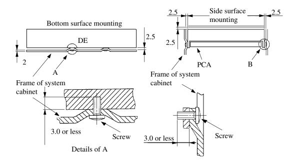
Figure 3.2 Mounting frame structure
